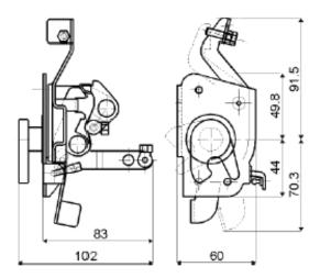
The P62 Lock is similar to P70, except that it contains a latch/logic to work in conjunction with the P61 Drivers Door Handle providing a drivers door solution.
