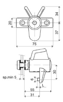
The P76 Sliding Window Lock is designed to secure sliding windows and releases easily by squeezing the 2 tabs together which raises the pin out of window hole. It is easy to install and fasteners are included.
