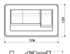
The P119 Locking Handle is a standard locking door handle for use with entrance and compartment doors. Available in three different operational models: Manual, pneumatic, and electric (operated with an electric actuator). Available with up to 40 different combinations utilizing the patented "JOK" (Just One Key) system, where the key and locking tumbler are supplied separately from the handle.
