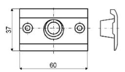
The P301 Pin Strike is designed for use in pantograph style luggage doors to retain the bottom of door, allowing the top to tip -in and secure.
