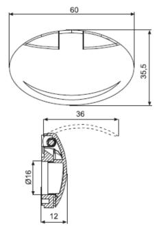
The P144 Lock Cover is the perfect choice for battery compartments, maintenance hatches, or any other exterior door. Its polyamide fiberglass construction offers superior weather protection, while its stainless steel pin and spring ensure a lifetime of reliable use. Mounts easily over any lock with two self-tapping screws (not included).
