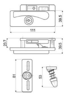
The P117 Locking Pin is a pin style lock designed for bottom hinged interior overhead compartments and is available in both locking and non-locking versions.
