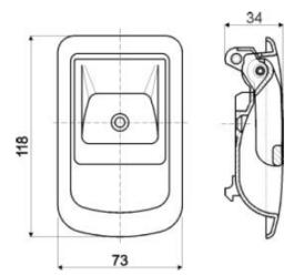
The P246bis Door Handle is the ideal choice for any interior door application. Constructed from durable PA6 plastic, the P246bis Door Handle is also UV-resistant so it is protected from the elements. Locking hardware and latches are also available for a complete installation.
