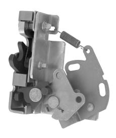
This latch and linkage system is intended for occupant or exit/entry doors for recreational vehicles including motor homes and travel trailers and specialty vehicles including ambulance, fire/rescue and off-highway vehicles (light duty) that require compliance to FMVSS 206 standards. The flexible design allows for internal or external door mounting and provides automotive logic function with remote activating handles.
