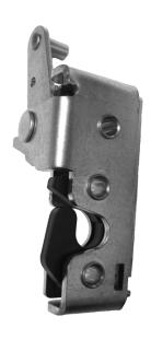
This slimline heavy duty latch module is designed for medium to heavy-duty vehicle entrance and rear door applications. It features a proven single rotor latch design, high strength 8 gauge (4.2mm) front mounting plate and robust straddle mount release lever. The slim design mounts into 2.00" (50.8mm) doors and retrofits competitive single rotor wedge style rotary latches
