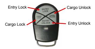
The FOB transmitter and receiver are shipped programmed. After making all necessary wiring connections (see Appendix B, page II for wiring information), the **e-FOB** system will function as shown.
