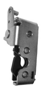
This latch is designed for medium to heavy-duty vehicle entrance and rear door applications. It features a proven single rotor latch design, high strength 8 gauge (4.2mm) front mounting plate and robust straddle mount release lever. The slim design mounts into 2.00" (50.8mm) doors and retrofits competitive single rotor wedge style rotary latches
