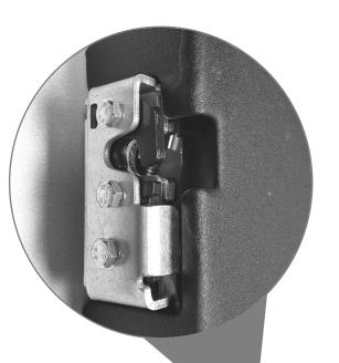
This heavy duty, pre-engineered door module was updated to provide expanded functionality. Providing automotive-like functionality in a low profile, easy to install one-piece module, it is now available with a rotating lever exterior handle and a second remote latch. Featuring Tri*Mark*'s 050-1600 Heavy Duty Latch, it allows power locking and is compliant to FMVSS206 (ECE R11) strength requirements.
