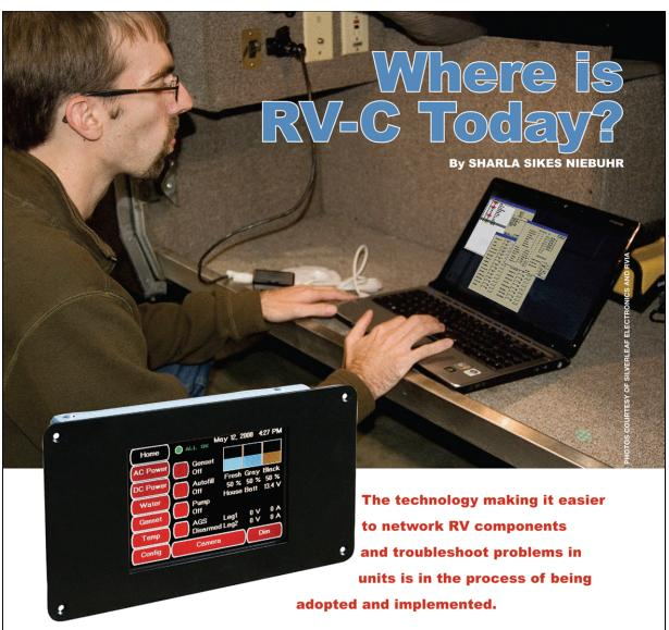
One of the advantages of RV-C is that it makes it possible to operate RV components such as an RV's awning, generator and hot water heater remotely, from one location.
