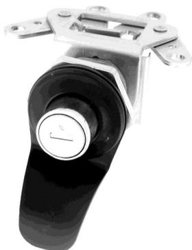
This new product is a redesign of our popular 040-0400 Push Button Center Control for lift gates, access panels, compartment and baggage doors. It features KeyOne™ Plus keying in a push button actuation and a two point bellcrank linkage.
