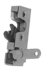
This compact single rotor latch is designed for light to medium applications for on or off-highway entrance doors, compartments and access panels. It features a variety of trip levers and mounting axles for ease of mounting and application and is FMVSS 206 compliant.
