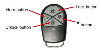
The FOB transmitter and receiver are shipped programmed. When the OEM has installed your **e-FOB** system, it will function as indicated below.
